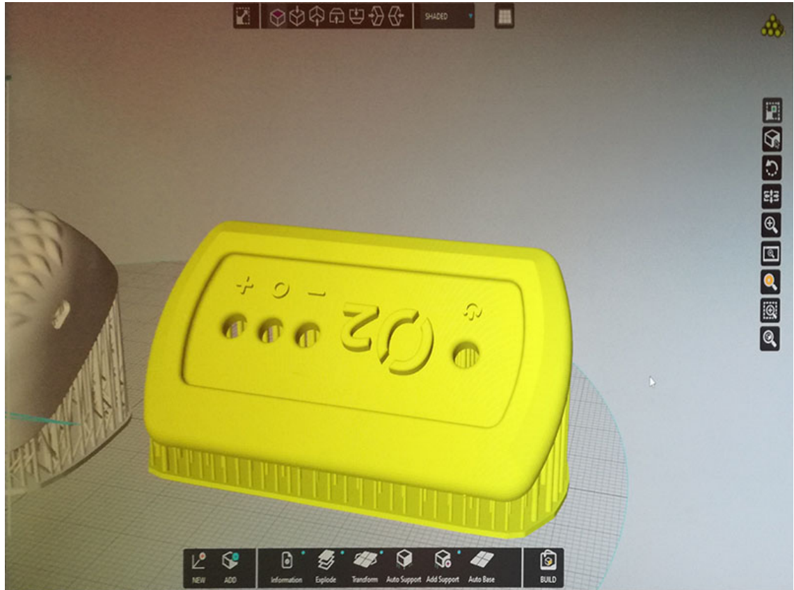
Fig. 5. 3D printing the Zero2 shells using a SLA printer.
